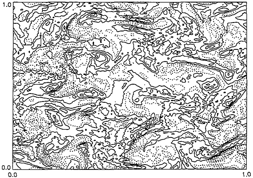
Figure 2. One realization of the stochastic process \omega_{\lambda,\mu} = \delta\psi N_{\omega}^{\lambda,\mu} defined by the master equation (14). The initial condition has been drawn from the initial ensemble defined by equations (59) and (60). The figure shows the vorticity contours at time t = 3 . The parameters are the same as in figure 1.
